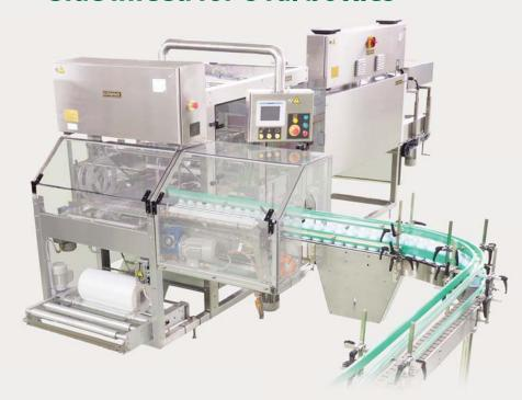
Autopack SLO CMOS is a Continuous Motion Overlap Seal bundle shrink wrapper with side infeed designed for handling oval bottles or shaped containers. With a maximum speed of 45 cycles/min, it is Autopack's fastest machine and among the world's most compact overlap seal machines.
