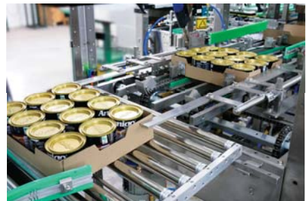
Direct connection to Shrink Wrapper
