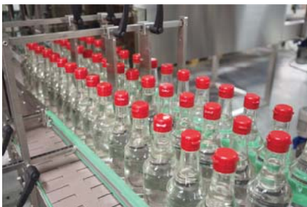
Multi lane infeed conveyor
