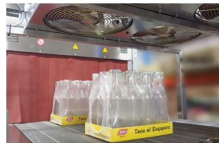
Cooling fans at outfeed
